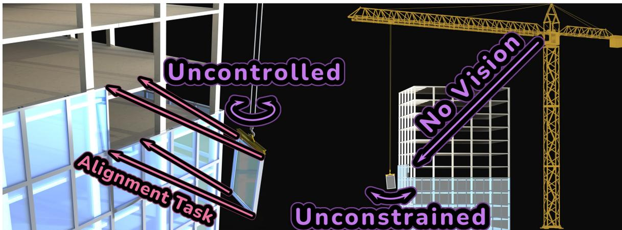
**Figure 2.5:** Render of the alignment task in the conventional direct UCW installation methodology, depicting the key limitations.
