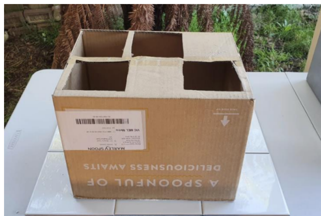
Figure B.5: The cardboard box provides a barrier to shield the fuel grains from the surrounding elements as they cool. The slots on the top of the box is used to help keep the fuel grains standing vertical as they cool.
