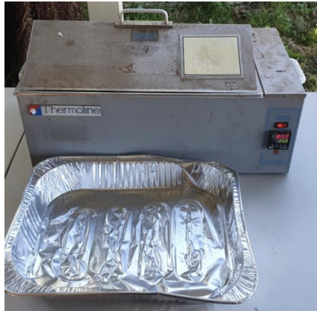
Figure B.2: Water bath preheating stage. The equipment is started prior to use up to 80 degrees Celsius. An important note is to ensure the lid remains enclosed to speed up the rate of heating.
