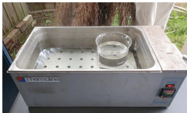
Figure B.4: Image of the paraffin wax heating process. The step utilised the water bath to reach the set temperature needed to melt paraffin. Depicted is the paraffin in its molten state.
