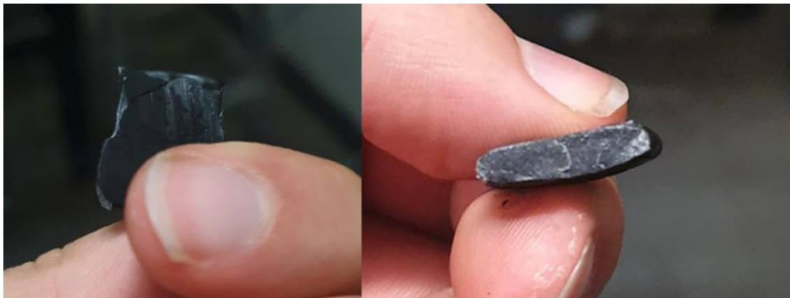
Figure 5.15: Hardened paraffin wax sample post gyroid fuel grain hot fire.
