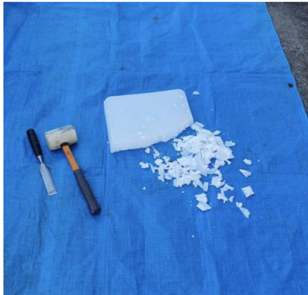
Figure B.1: Image taken of the break-down of paraffin wax slabs in process to achieve smaller more easier to melt portions of wax.
