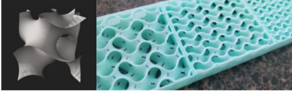
Figure 4.1: (Left): Single gyroid unit cell. (Right): 3D printed gyroid samples at different infill percentages.
