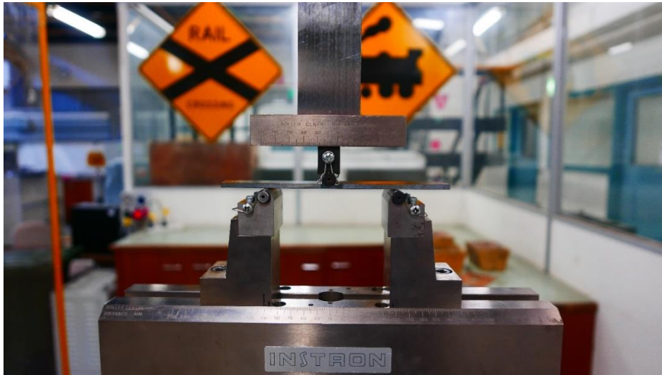
Figure 3-8 Three point bend test setup for a unidirectional specimen undergoing static loading
