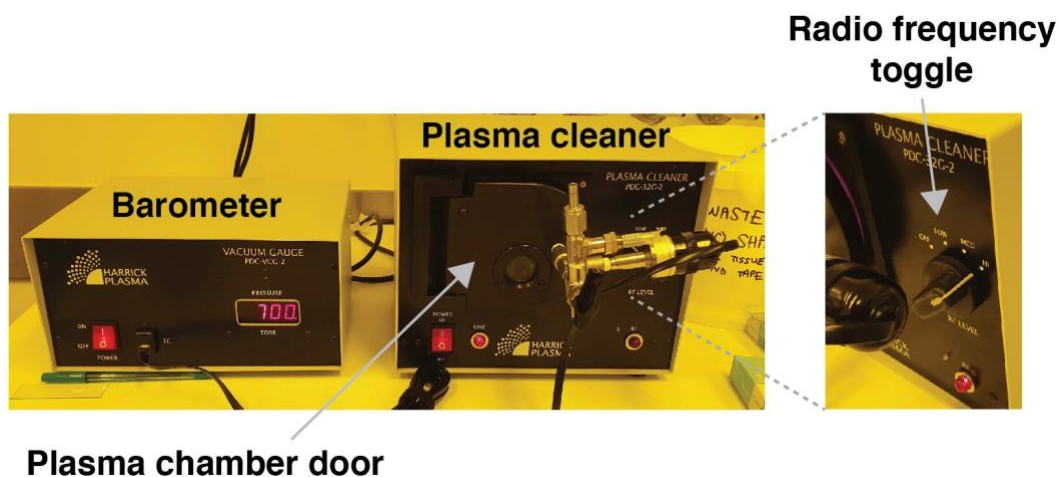
Fig.4 Plasma cleaner set-up. The plasma cleaner is connected to an electronic barometer that monitors the plasma chamber pressure with pressure readings displayed in units Torr. The plasma chamber door seals the chamber to allow the chamber pressure to drop upon activation of the vacuum source. When the desired pressure is achieved, the plasma cleaner is activated via a radio frequency toggle with four settings: “off, low, medium and high”; toggle setting shown in the right image is set on “high”
