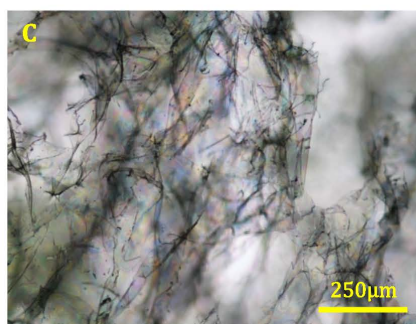
Fig. 4. (A) The effect of freezing rate (initial freezing at -20^{\circ}\text{C} , -80^{\circ}\text{C} , and -196^{\circ}\text{C} ) on the FSC in deionised water. Optical microscopy illustrating the effect of freezing at (B) -20^{\circ}\text{C} (C) -80^{\circ}\text{C} , and (D) -196^{\circ}\text{C} on the morphology of nanocellulose foams.
