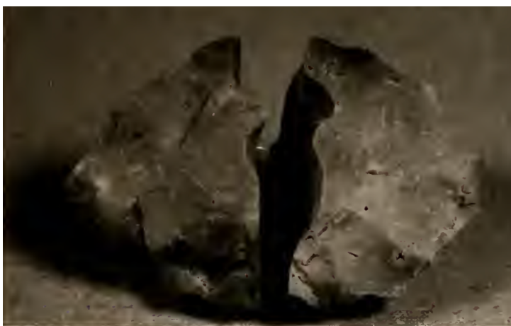
Figure 10. Crenated fracture (after Purdy 1971:55).
