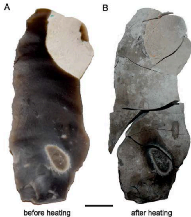
Figure 7. Deep surface cracks on flint artefacts following temperatures above 650 °C (after Fiers et al. 2021: 40).
