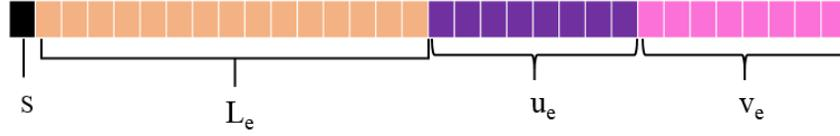
Figure 2.2.6: 32-bit LogLUV bit distribution
