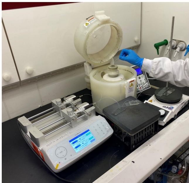
Figure S4: Picture of the fabrication setup located in the fume hood (from left: dual syringe pump with preloaded NiO x dispersions, microfluidic mixers, spin-coater and annealing plate). The computer-controlled syringe pump triggers the simultaneous push of two syringes which are preloaded with equal amount of thoroughly mixed and ultrasonically shaken dispersions, the tubing is connecting both syringes to the inverted-multistage Tesla valve and pushes the solutions through it (the channels inside of the Tesla valve have micropillars (1-3 μm), the Tesla valves can be connected in series for better mixing or the tube can be directly positioned above the substrate. The aliquoted amount (typically 50 to 100 μL) is being deposited and the spin-coater with pre-programmed speed and time begins the spin-coating. The substrate is subsequently removed from the vacuum chuck and placed on the hot-plate.
