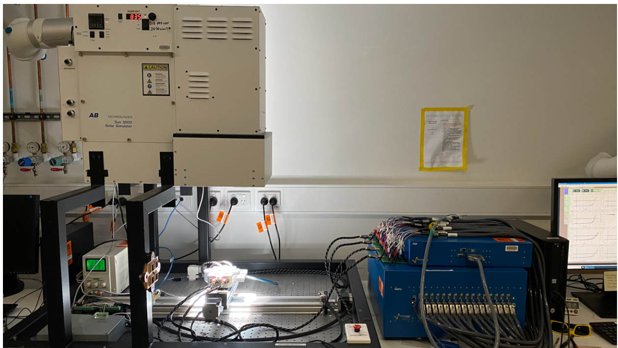
Figure 43: Digital photograph of operating high-throughput characterization setup used in Renewable Energy Laboratories at Monash University built by author. More details can be found in Chapter 7.
