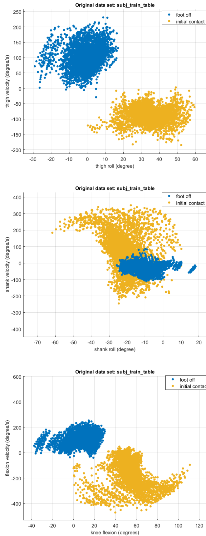
Figure 5.4: Scatter plot of the original data for the two 5-sample wide transition outputs (initial contact and foot off) during stair ascent with axes presenting the angle and velocity of each attached body (top: thigh, middle: shank), and the presumed joint (bottom)
