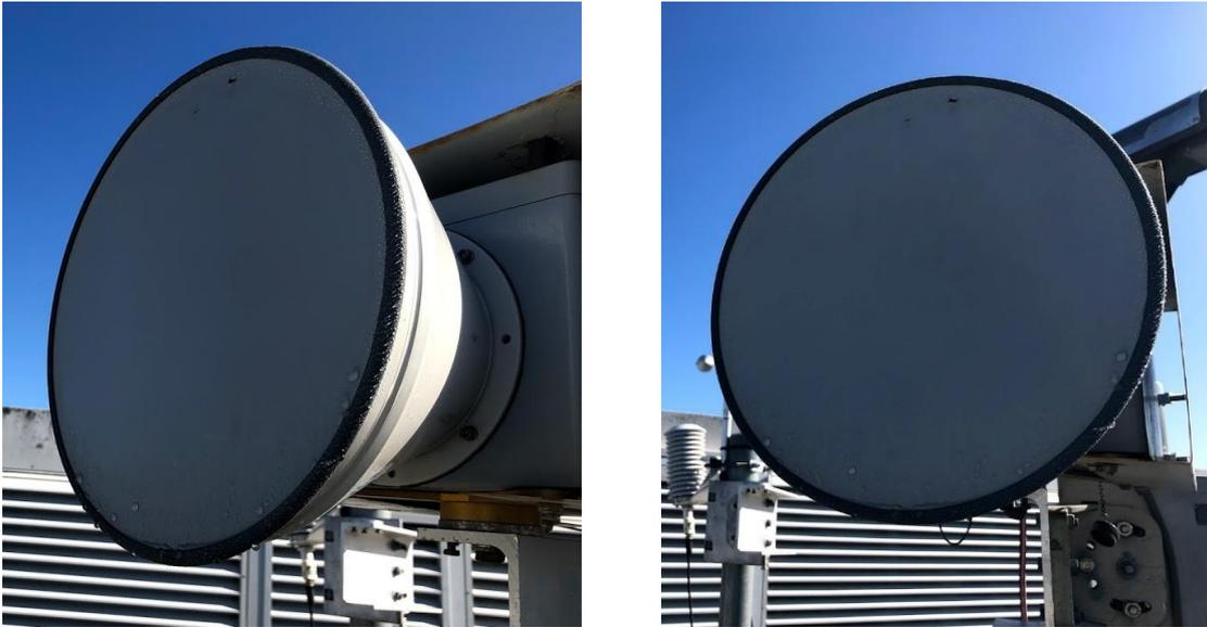
**Figure 4-19: Photograph of the receiver antenna just after receiver antenna sprayed with water during the wet antenna experiment. Water droplets formation was observed on the antenna film.**
