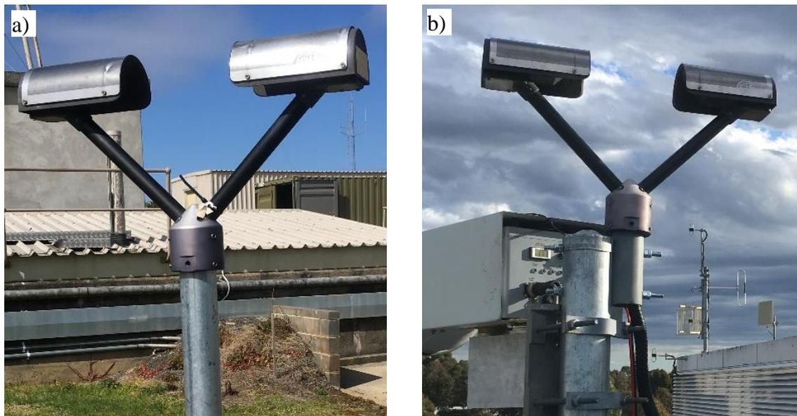
**Figure 3-6: The OTT PARSIVEL1 disdrometers installed at each end of the experimental link path. (a) Disdrometer installed at the Melbourne Water Mount View reservoir and (b) Disdrometer installed at Lakeside Driver, Burwood.**
