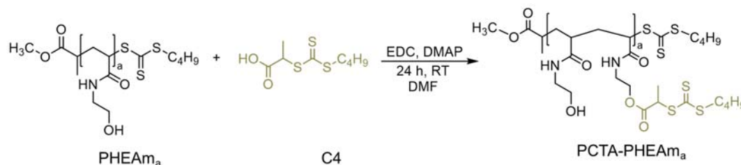
Scheme 2.3 Representative reaction scheme of polyCTA backbone formation
