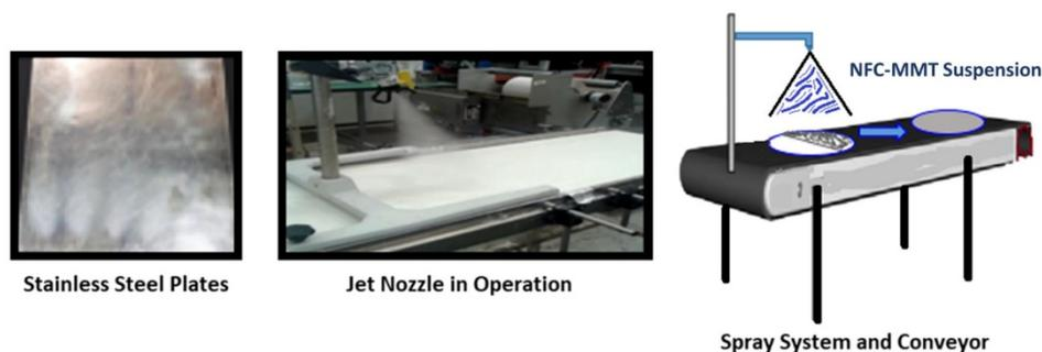
**Fig. 1** Experimental setup of spray coating system
