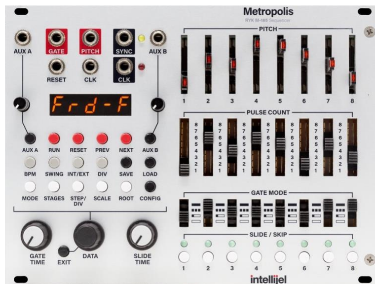
Figure 17. Metropolis sequencer Eurorack module by Intellijel
