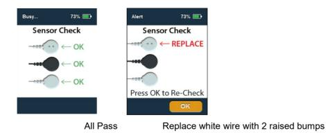
3. If a sensor needs to be replaced, and at least 30 minutes has passed since sensor pad application (Step 1), simply remove, discard, and repeat the steps above using a fresh sensor pad. Never re-use a sensor pad.
