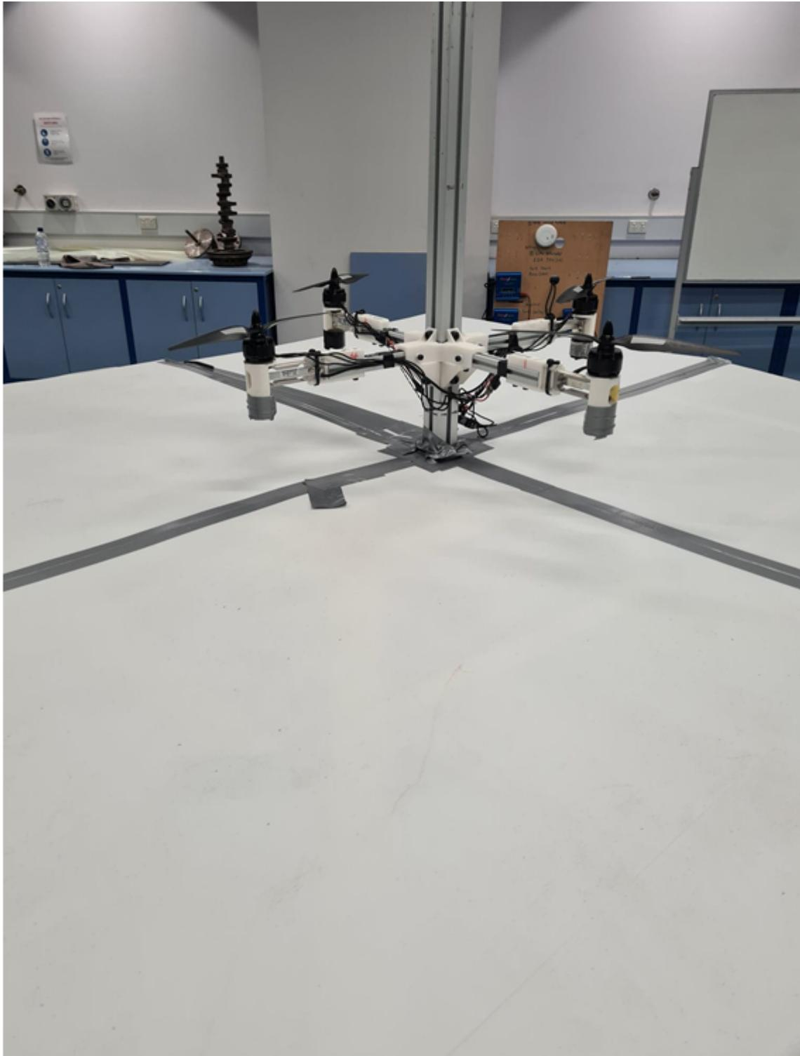
Figure 4.15: Setup of the  $OS_g$  case. 16 tripod were evenly distributed at the bottom of the corflute panel to support the structure.
