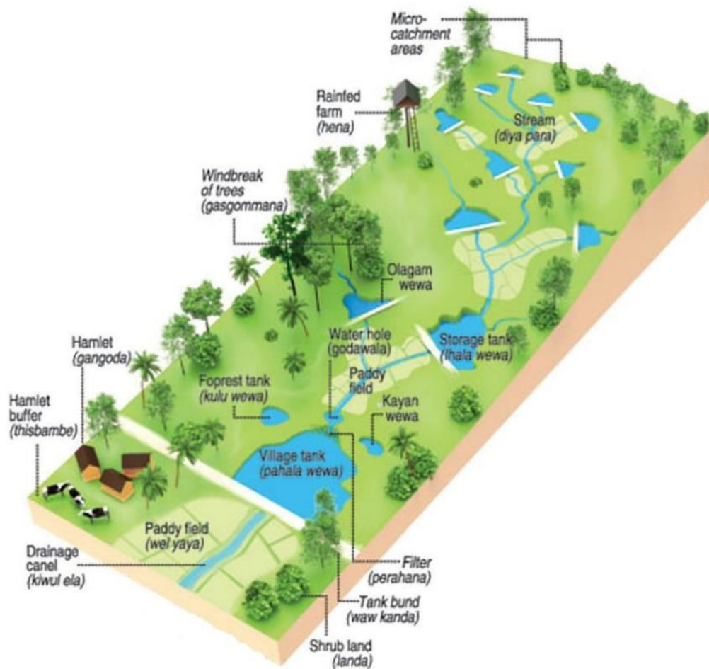
Figure 4.3. This is an image of the layout of the Tank Cascade System that existed in Sri Lanka since at least 1200 BC (Geekiyanage & Pushpakumara, 2013). As can be seen, the circulation of water is mapped to suit the immediate geographic contours of the landscape.
