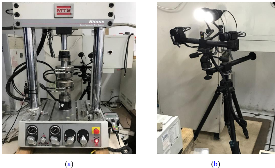
Figure 3-2: Experimental facilities: (a) MTS858-Bionix test machine with the Flex-Test 40 system; (b) DIC system.
