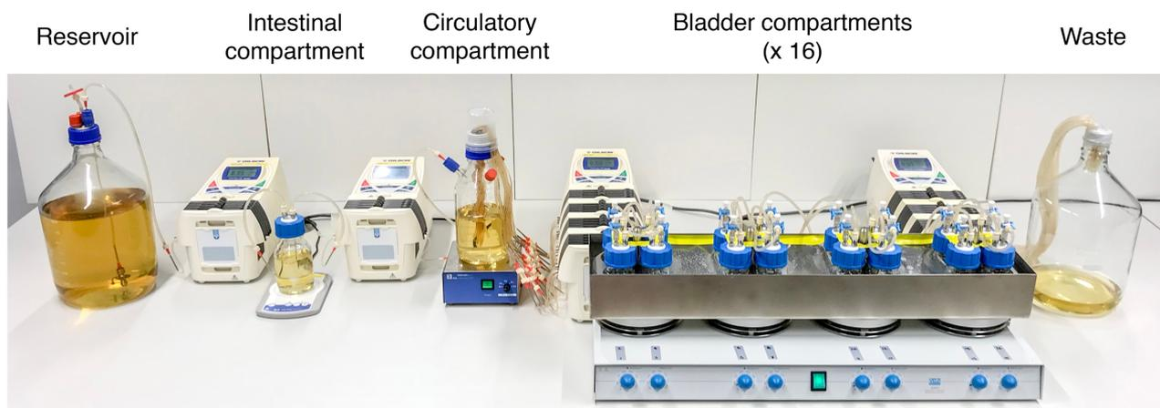
**Figure S1. Bladder infection *in vitro* model design**
