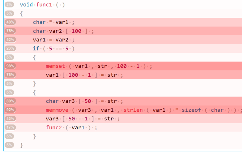
Figure 5.8: Example heat map that represents the vulnerable relevance probabilities over the given source code.
