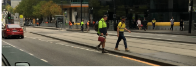
c. ROW B.3 tram tracks longitudinally-separated by non-mountable barrier kerb (note: jaywalking pedestrians)
