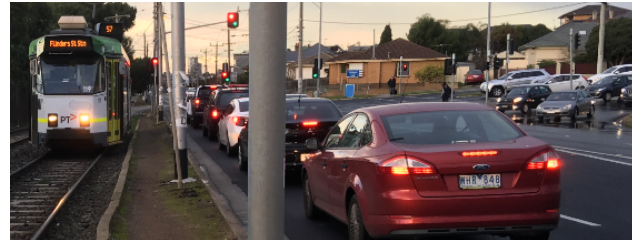
b. ROW B.1 (side-running) longitudinally-separated tram
