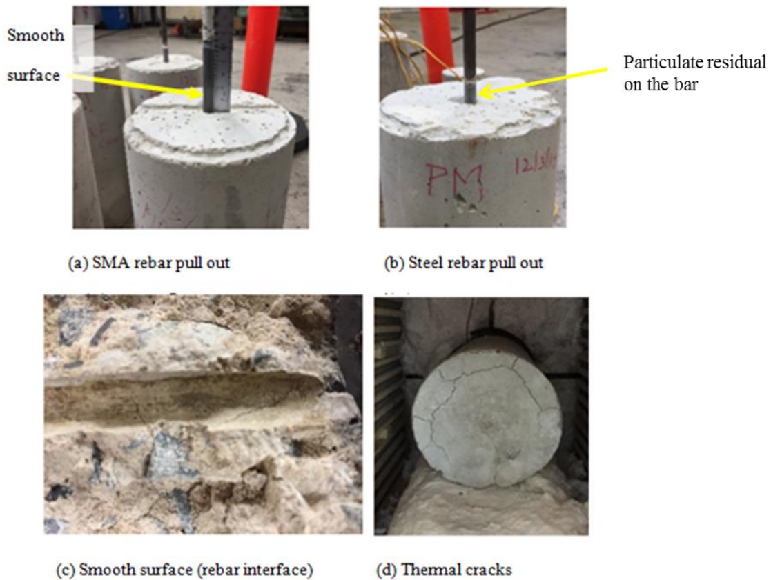
Figure 3.51: Failure Modes: Pull out test under high temperature
