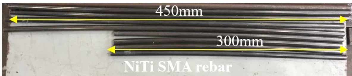
Figure 3.14: Cut SMA rebar of length 450 and 350mm
