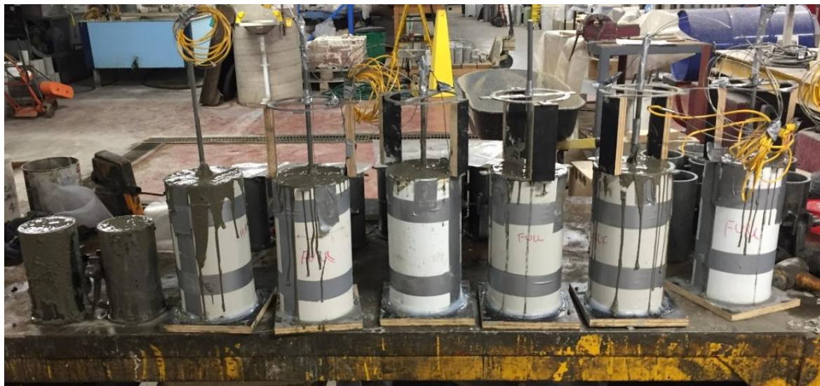
Figure 3.18: Cast test specimen with SMA rebar and thermocouple.
