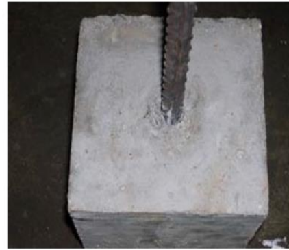
Figure 6.14: Bond-slip response pull-out test (Apparao et al. 2002)
