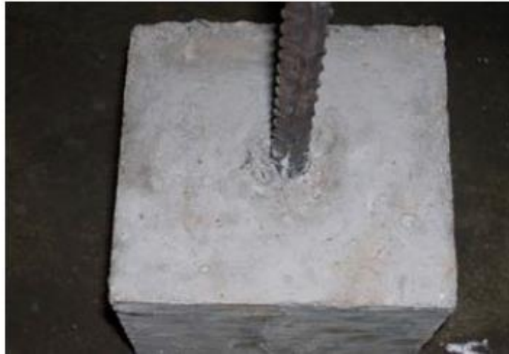
Figure 4.14: Typical specimen for pull out testing (Apparao et al. 2002)
