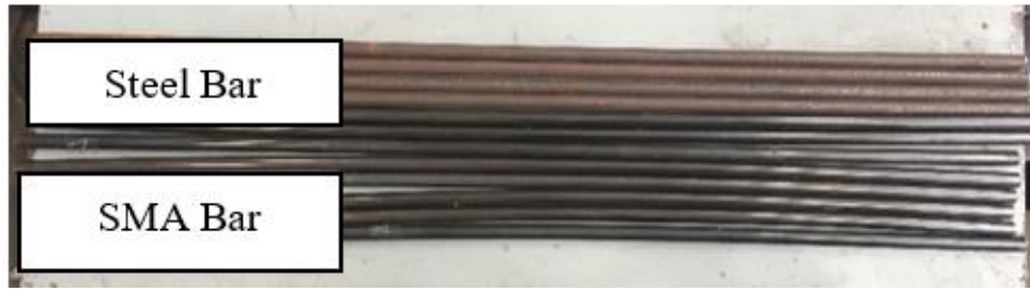
Figure 3.6: Steel and SMA rebar 10mm diameter
