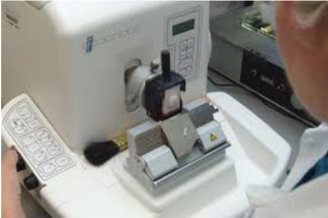
Figure 2. 2: Paraffinised Tissue Block Slicing Process
