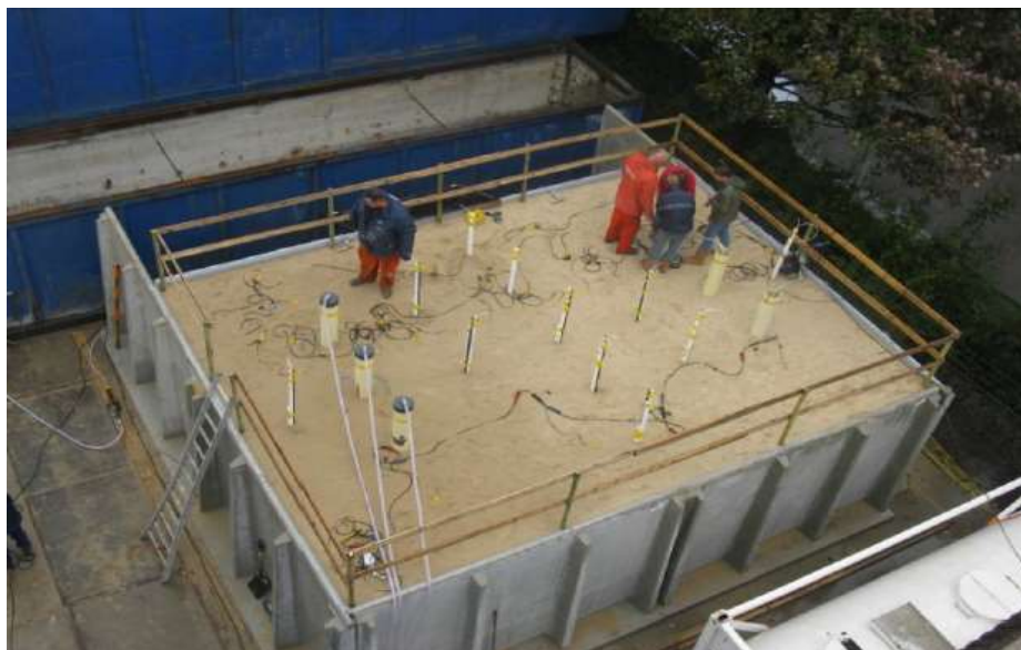
Figure 1.5. Setup for large-scale biogrout experiment to strengthening 100 m 3 sand (Van Paassen et al. 2009; Van Paassen 2011).
