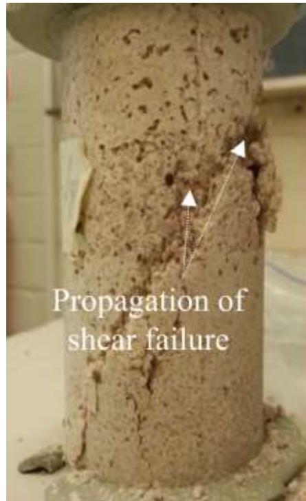
Figure 5.6. Typical failure pattern of a bio-cemented coarse sand column.
