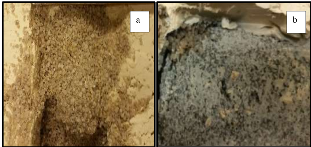
Figure 8.4. Clay ingress into the column: a- in-situ bio-cemented sand column; b- ex-situ bio-cemented sand column.
