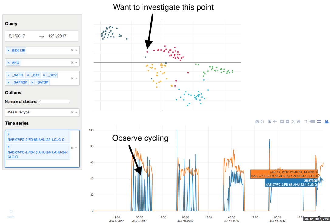
Figure 6: Control valve short cycling. One of the CCV points (red) is far from the others. Selecting this point quickly reveals short cycling occurring in the anomalous point. Another point from the main cluster has been selected to illustrate what CCV readings from a normal point should look like.
