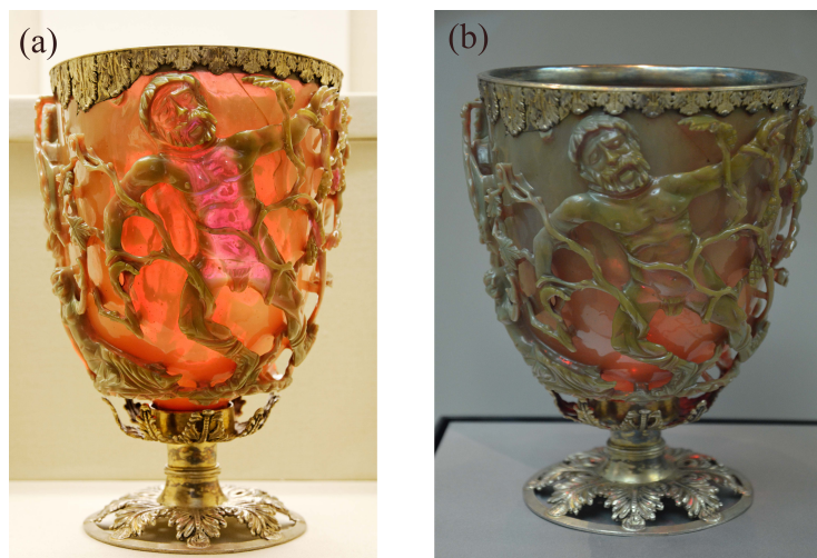
Figure 2.1: This figure shows the Lycurgus cup, which is made by glass embedded with noble MNPs. The glass appears red and translucent when illuminated from inside of the cup (a), and green and opaque when illuminated from outside (b).
