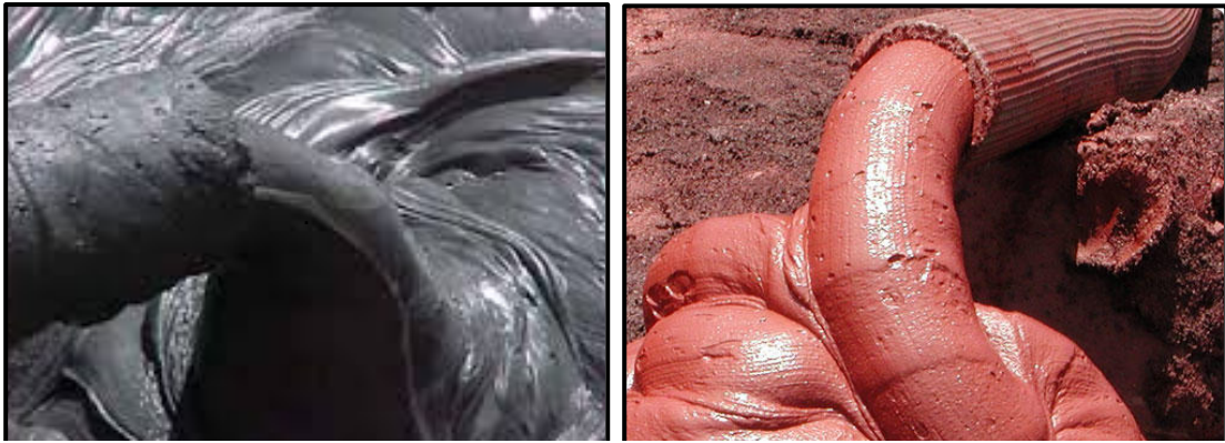
Figure 2.2: Coal (left) and copper (right) tailings depicts the highly viscous nature of the fluid V.Boger (2013).
