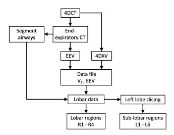
FIGURE 4.7: Flowchart showing the post processing tasks for the 4DCT imaging data and analysis of the regional distribution of tidal volume ( $V_T$ ) and end-expiratory volume (EEV).
