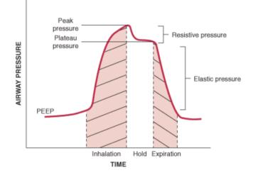
FIGURE 2.3: Airway pressure versus time during constant flow, volume-control mechanical ventilation. The inflation-hold manoeuvre (typically 1 second) enables the plateau (alveolar) pressure to be measured. The resistive pressure is the pressure required to overcome airway resistance. Elastic pressure is the pressure required to overcome the elastic recoil of the lungs and chest wall (Porter, 2020).
