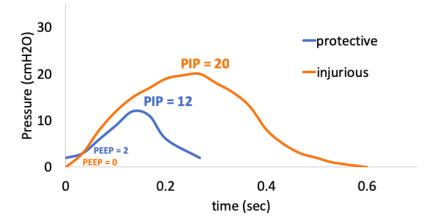
FIGURE 4.2: A representation of pressure (relative to atmosphere) versus time showing the two ventilation strategies used in the studies: protective (225 breaths per minute) and injurious (100 breaths per minute).
