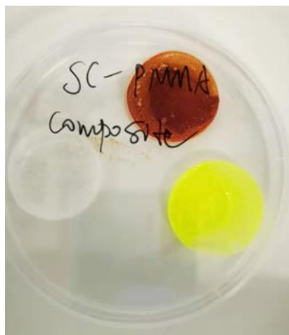
Figure 2-5. Photo of the SC-PMMA composite material. The white, yellow and brown disks consist of the \text{CsPbCl}_3 , \text{CsPbBr}_3 and \text{CsPbI}_3 SCs-PMMA composites, respectively.
