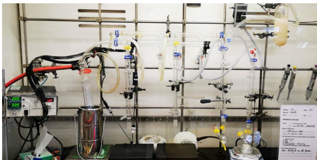
Figure 2-1. Schlenk line used in typical Cs-precursor and \text{CsPbX}_3 synthesis.
