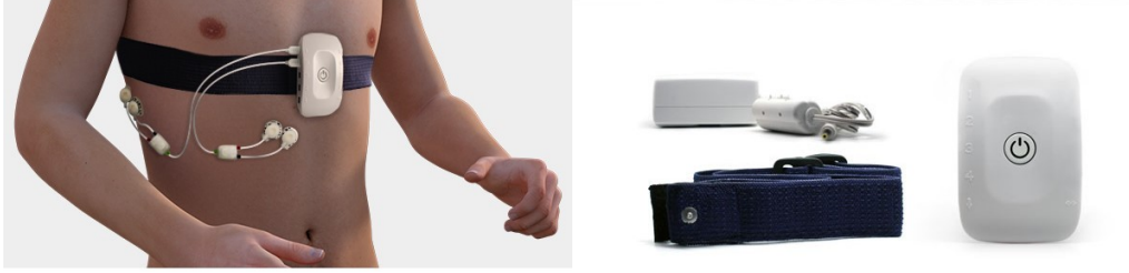
Figure 2.2: Placement of the RespiBAN on human torso.
