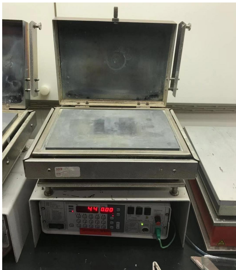
Figure 2.4 The digital photograph of the titanium hot plate with a PID temperature controller.
