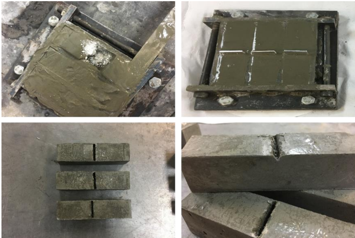
Figure 14: Casting of cement paste specimens with the artificial notch.
