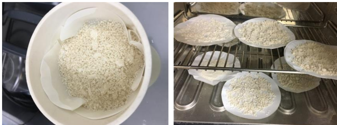
Figure 11: Filtration and oven drying of microcapsules (EPU)
