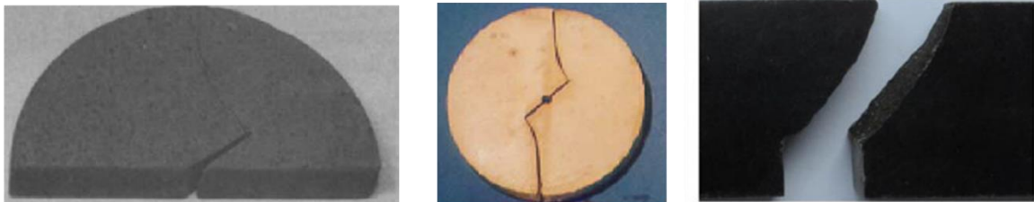
Figure 2.0-7. Mode I and mixed mode fracture patterns of rocks in (a) Notched semi-circular bending specimen (Lim et al. 1994); (b) CCNBD specimen (Al-Shayea 2005); (c). Notch four-point bending specimen (Wang et al. 2016).
