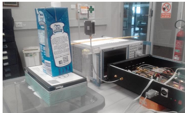
Figure 8.51 – Tagged milk carton detection using single patch antenna
