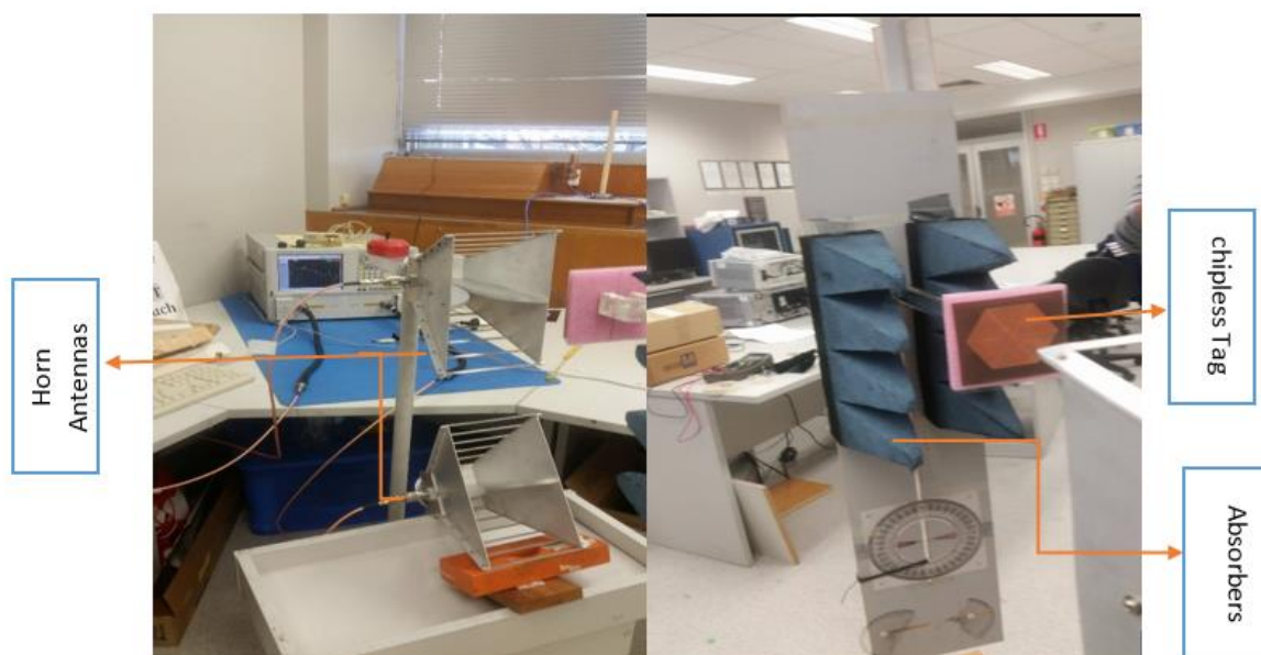
Figure 8.4 – (a) The experimental setup with two big horn antennas (0-18GHz) for S21 measurement using VNA (b) The hexagonal tag of 18-bits working in the range of 3-10GHz
