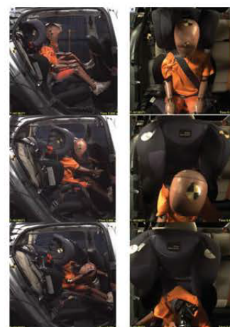
Figure 3. Test 2: Side view and top view of HIII 6-year-old in pos2, at 0 ms (first row), at 80 ms (second row), and at maximum head excursion at 103 ms (third row). Note the shoulder belt slippage into the gap between the shoulder and arm in the pictures in the right column.
