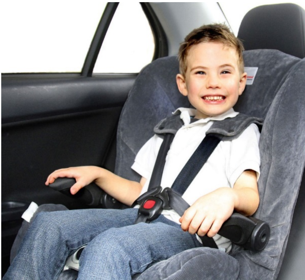
Figure 3. An exemplar of a typical FFCRS with a five-point harness, installed in a motor vehicle in Australia (Source: RACV, 2019)
