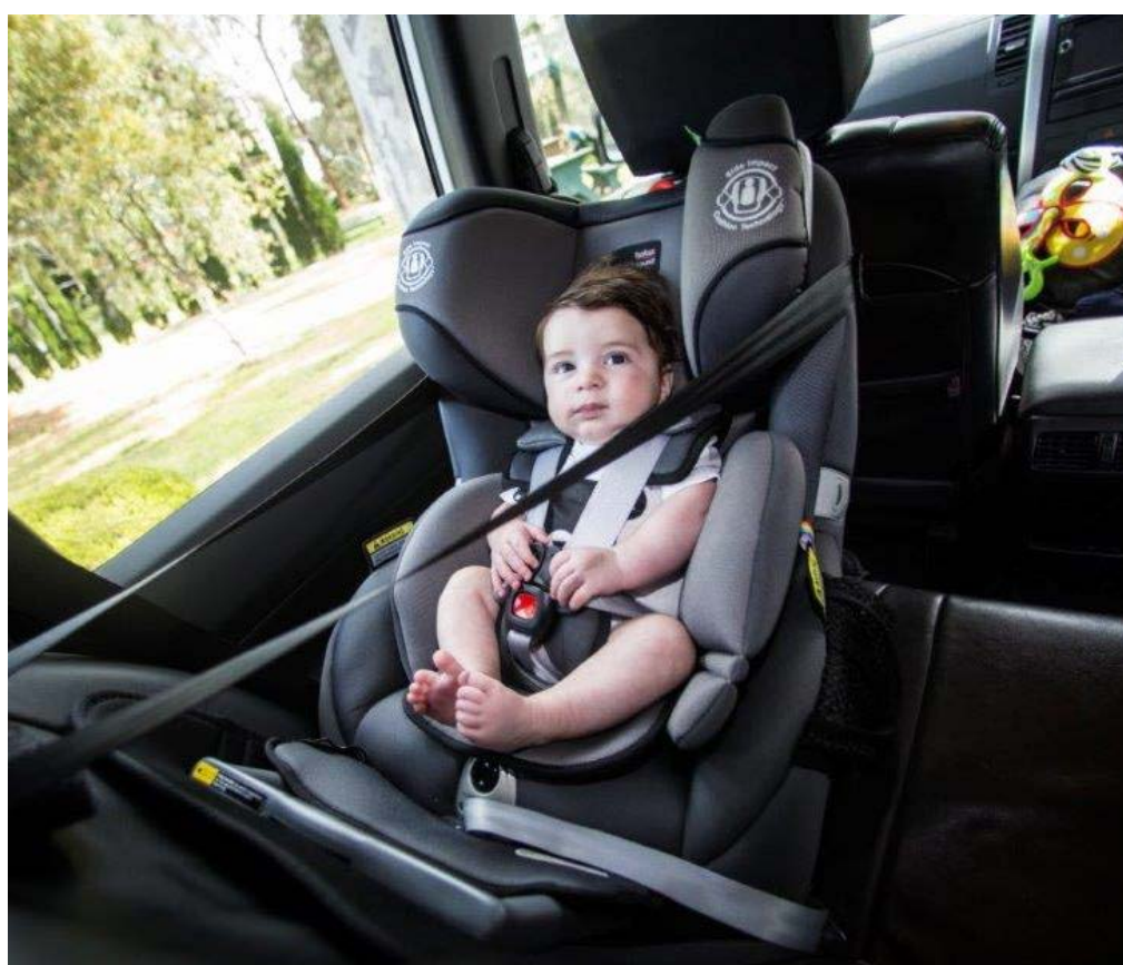
Figure 2. An exemplar of a typical RFCRS with a five-point harness, installed in a motor vehicle in Australia (Source: RACV, 2019).
