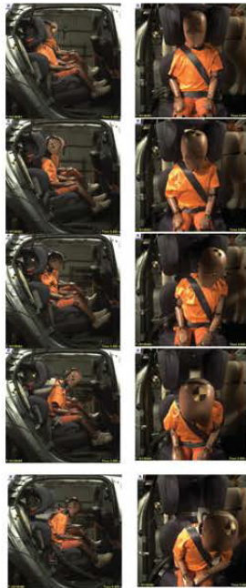
Figure 2. Side view and front view of the HIII 6-year-old in the 5 different positions tested, from top to bottom: reference, pos2, pos3, pos4, and pos5.
