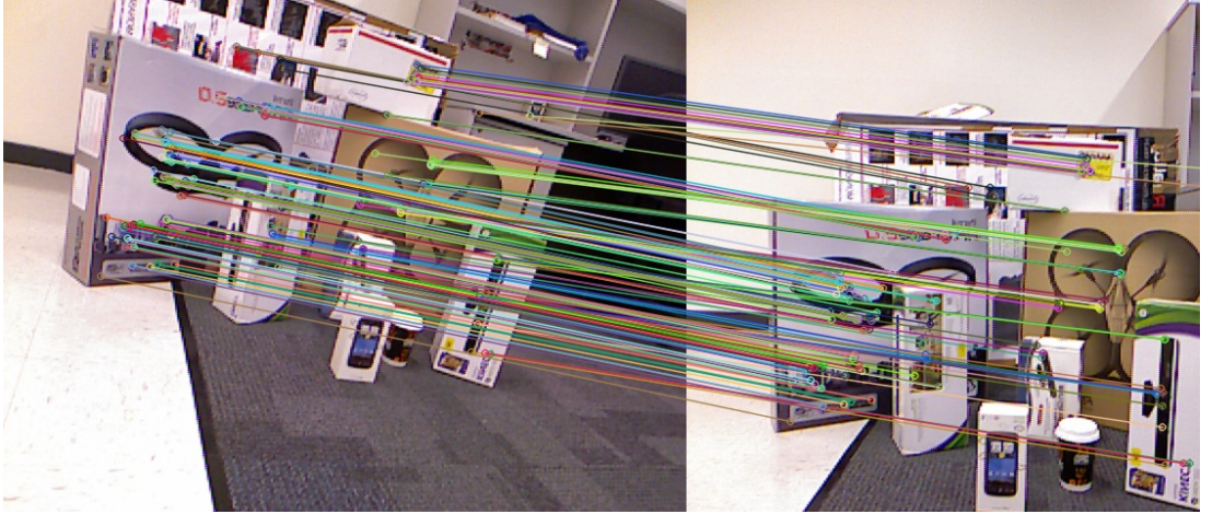
Figure 3.2: Matched ORB feature correspondences are filtered according to relevant depth information from two different RGB-D sensors
