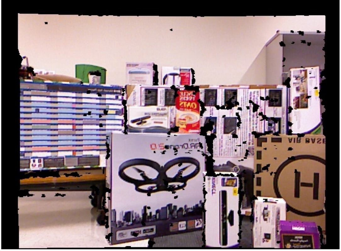
Figure 3.3: Integrated color and depth images from Kinect
