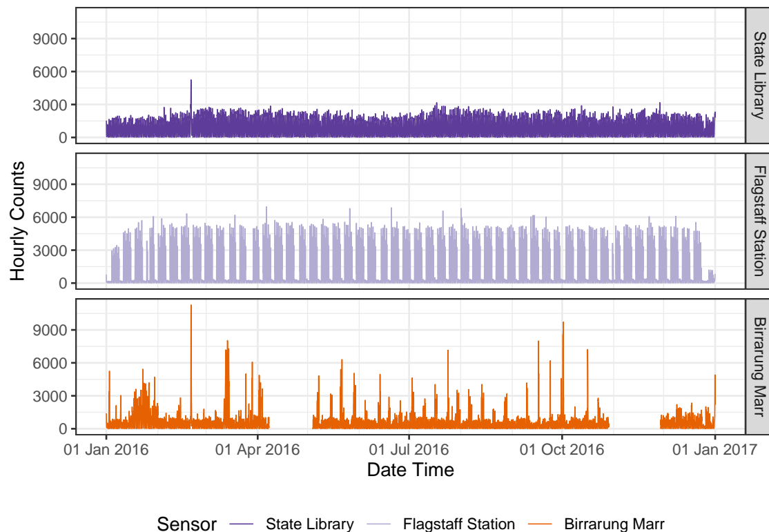
Figure 2.2: Time series plots showing 2016 pedestrian counts, measured by three different sensors in the city of Melbourne. Small multiples of lines show that the foot traffic varies at one location to another. The spike in counts at the State Library corresponds to the timing of the event “White Night”, where there were many people taking part in activities in the city throughout the night. A relatively persistent pattern repeats from one week to another at Flagstaff Station. Birrarung Marr looks rather noisy and spiky, with several runs of missing records.
