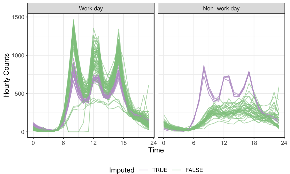
Figure 4.17: Examining the daily seasonality, relative to the work day vs not components, using faceted line plots. The imputation (purple) grasps the key moments (morning and afternoon commutes, and lunch break) in a work day, but is unable to build the non-work profile.
