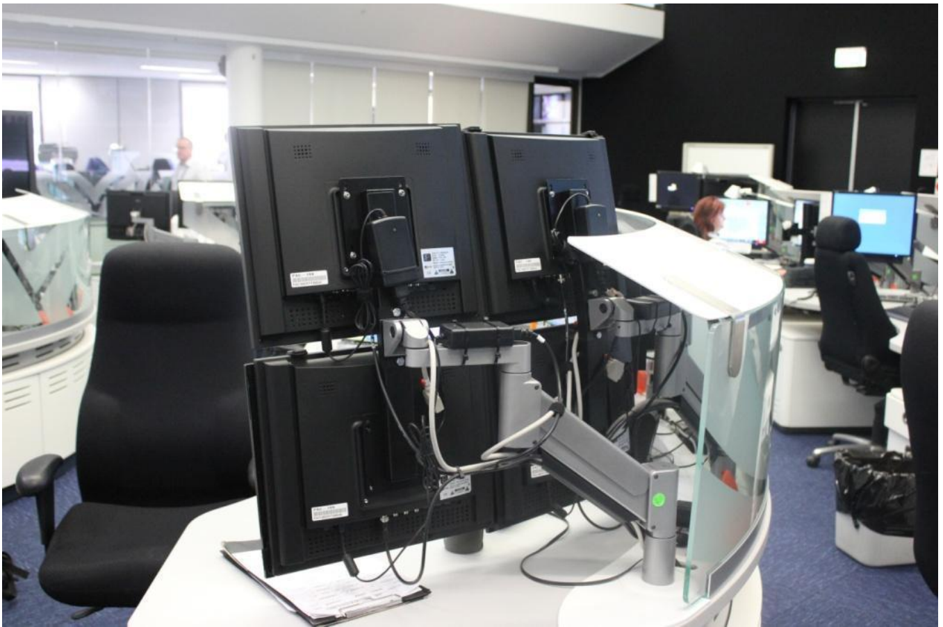
THE GAS ARTICULATED MONITOR ARMS ENABLE UP TO EIGHT MONITORS ON THE INDIVIDUAL WORKSTATIONS TO BE FINGERTIP ADJUSTED
