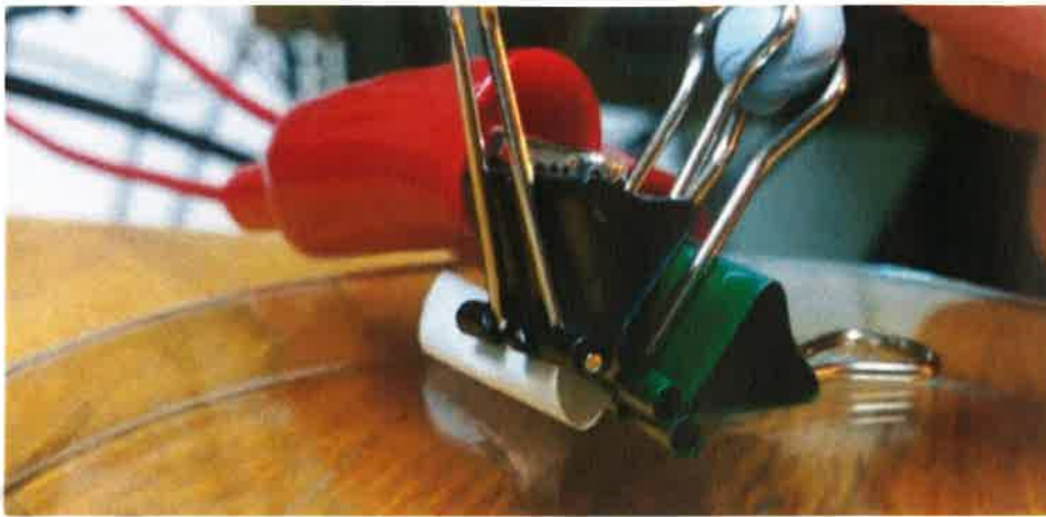
Figure 4. Electrical characterization setup for the AgNW-coated NF paper. Here, also an example for the bending is presented.
