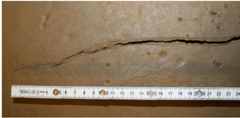
Figure 2.11. Surface depression on the crack tip (Tollenaar 2017).
