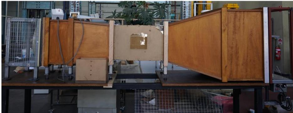
Figure 4.2. Wind tunnel body after fabricated.
