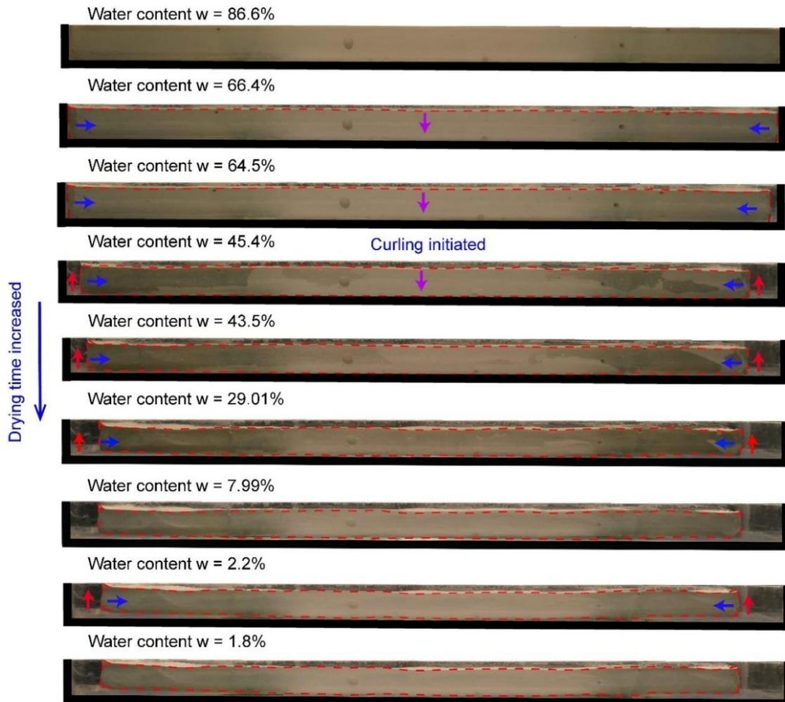
Figure 5.6. Shrinkage deformation and curling development of the Kaolin NY clay.
