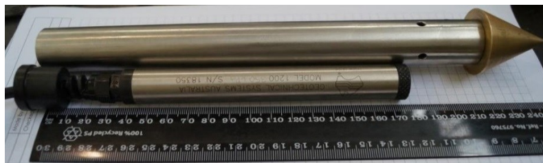
Figure 3.30. Vibrating wire piezometer and push-in cone
