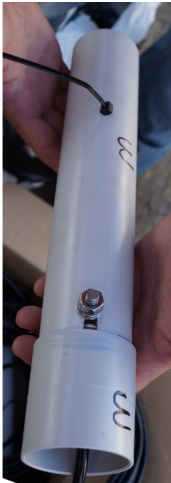
Figure 3.25. Inclinometer mounted in 50 mm diameter PVC
