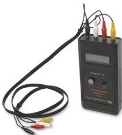
Figure 3.32. GSA - Model 9120 vibrating wire readout unit
