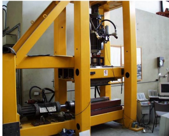
Figure D9. Large scale direct shear apparatus (from Haberfield et al. 2003)
