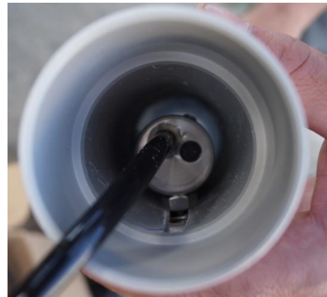
Figure 3.26. Top of mounted inclinometer
