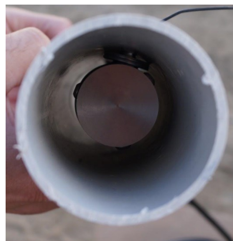
Figure 3.27. Base of mounted inclinometer
