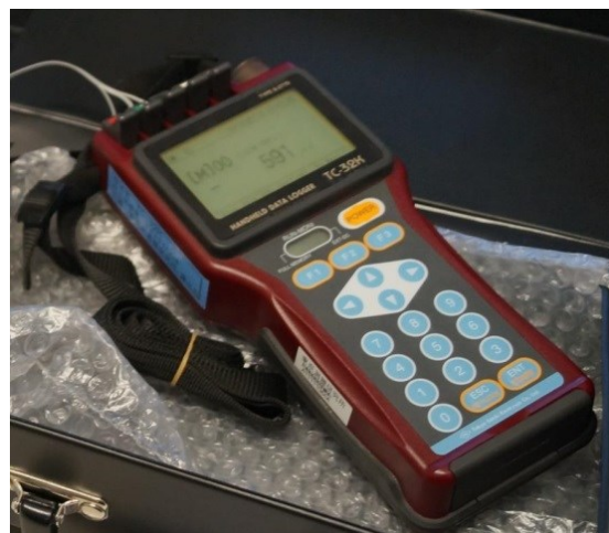
Figure 3.33. Tokyo Sokki Kenkyujo - TC-32K Handheld data logger
