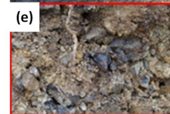
Figure 4.6. (a) Aerial image dated 3 March 2006, (b), (c) field observations of Historic Embankment Fill, (d) and (e) close up of fill material from Figure 4.6c.
