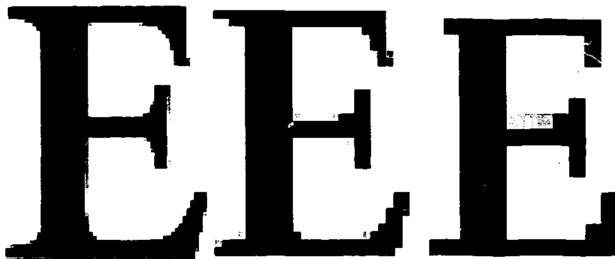
Figure 2.7 Sampling resolution example
