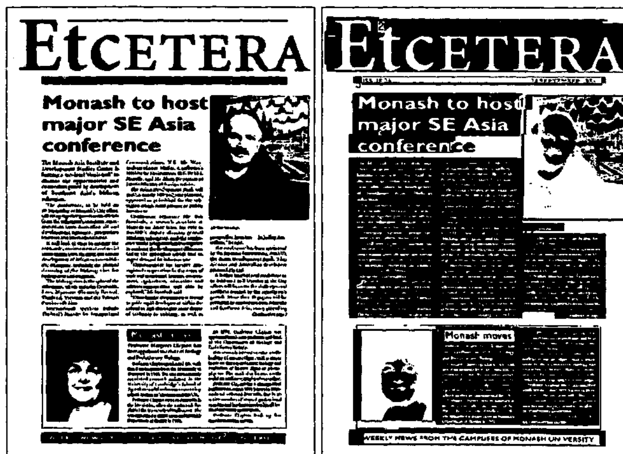
Figure 2.12 First segmentation phase example The newsletter on the left is segmented to produce the series of numbered text and non-text regions on the right.
