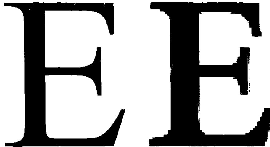
Figure 2.6 Continuous and sampled image example
