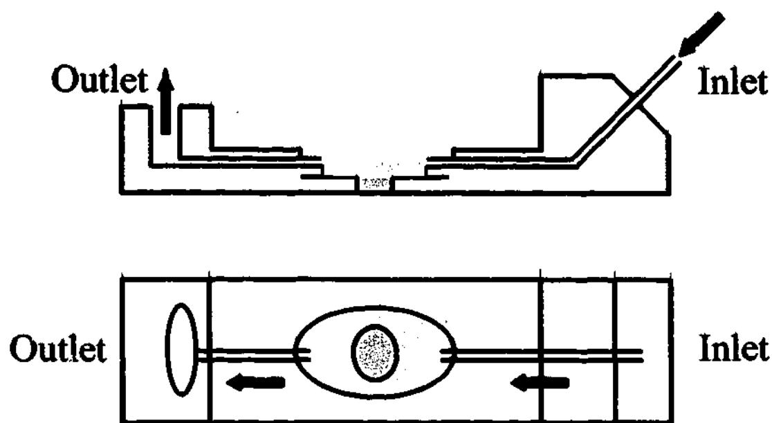
**Figure 2.6:** Schematic representation of the chamber that was used during fura-2 measurements from cells. The top panel shows a lateral view of the chamber. The lower panel shows a top view of the chamber. Improvements from the first chamber included an indented well for cells to sit in, and a smaller inlet tube to allow better control of solution flow into the chamber.
