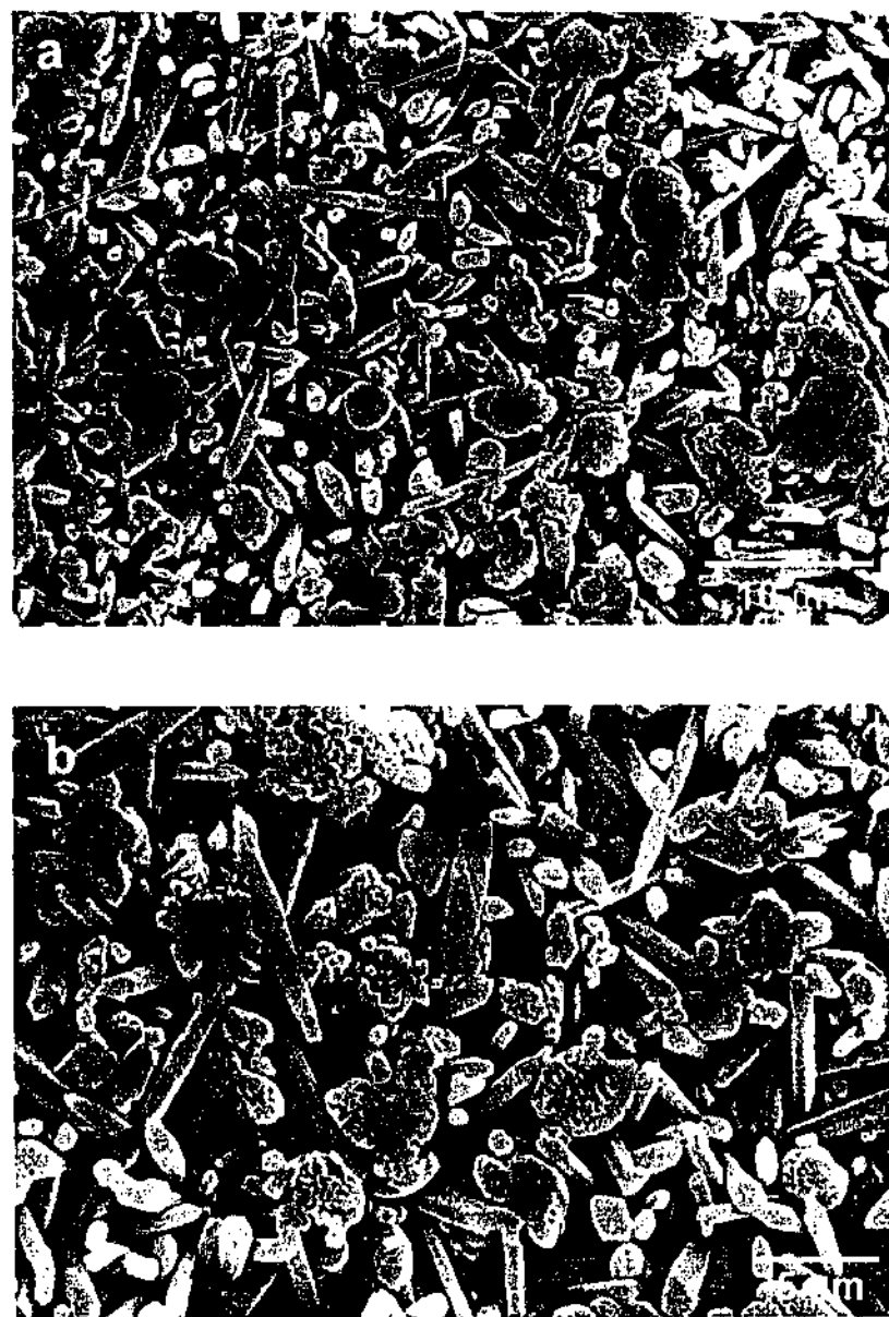
Figure 4.17. Secondary electron micrographs of polished and etched sections of composition 5025 sintered for 4 hours at 1800°C.
