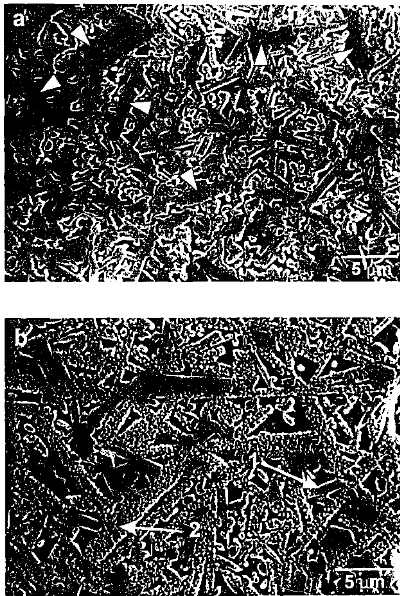
Figure 5.4. Secondary electron micrographs of polished and etched samples of (a) 2040 and (b) 2050, sintered for 2 hours at 1800°C. Polytypoid grains are arrowed in (a). Grains analysed by EDXS are labeled in (b).
