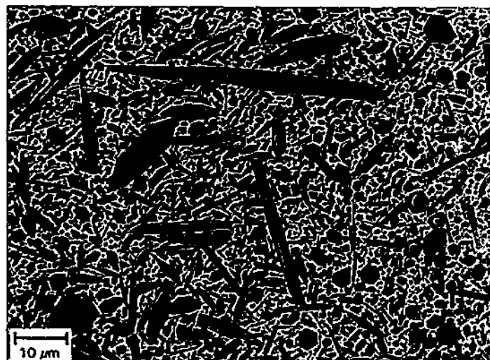
Figure 2.9. SEM micrograph of plasma etched \text{Si}_3\text{N}_4 ceramic. The microstructure consists of elongated \beta - \text{Si}_3\text{N}_4 grains embedded in a matrix of fine, equiaxed \beta - \text{Si}_3\text{N}_4 grains and grain boundary phase (Hoffmann 1994).
