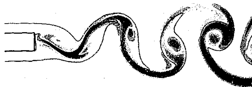
Figure 3.16: stream-wise vorticity field of the Mode S' instability ( AR = 7.5 , Re = 500 , \lambda = 1.0H ). The positions of the Karman vortices are highlighted by the contours of span-wise vorticity of the base flow at \omega = \pm 0.2 .
