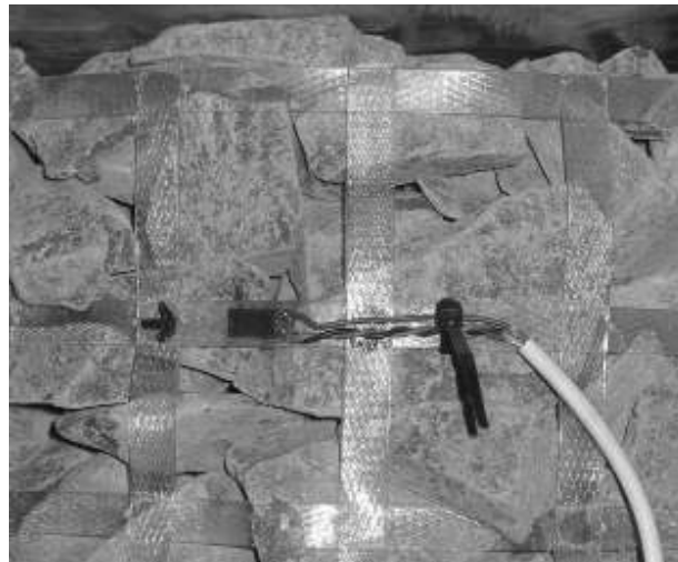
Figure 5.10: Strain gauge attached to the upper section of the encasement
