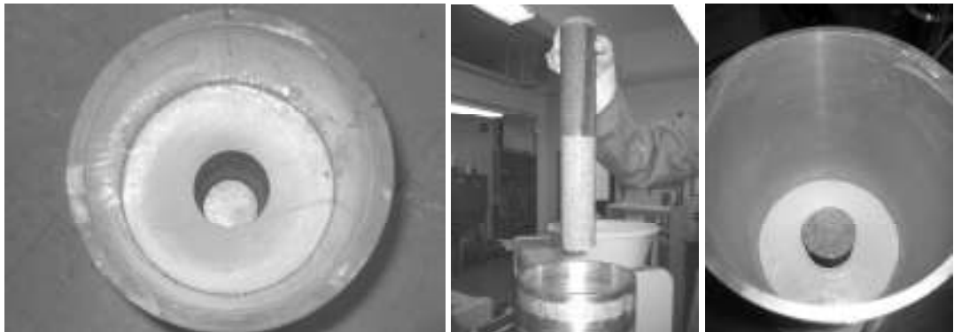
Figure 3.19: Installation of a frozen model sand column
