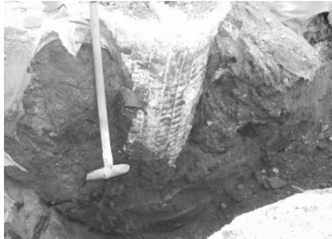
Figure 2.17: Excavated geogrid encased stone column
