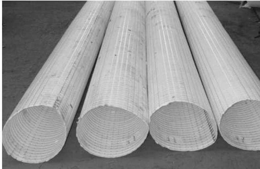
Figure 7.4: Prefabricated geogrid sleeves (welded)
