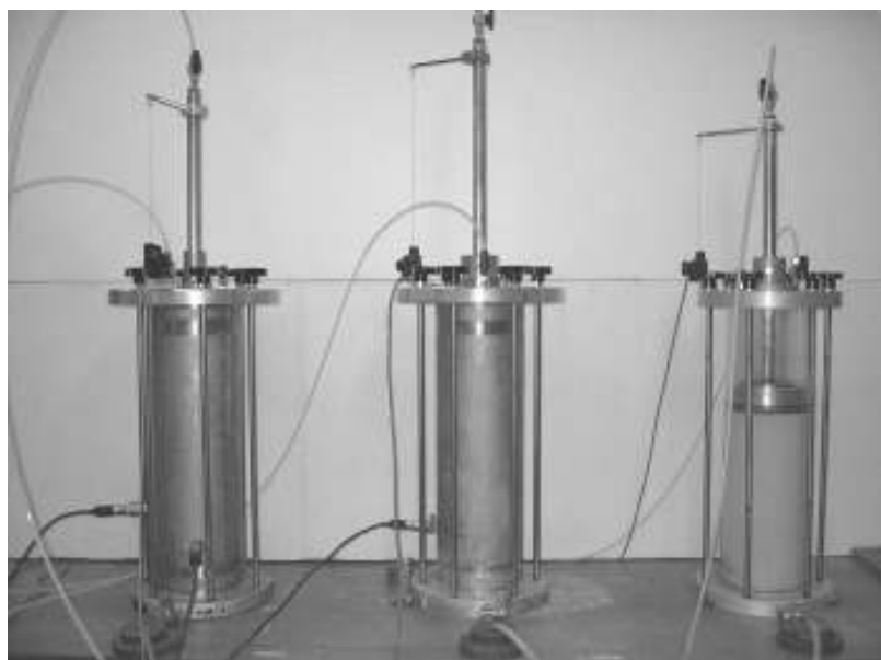
Figure 3.2: Consolidation cells used in model column testing
