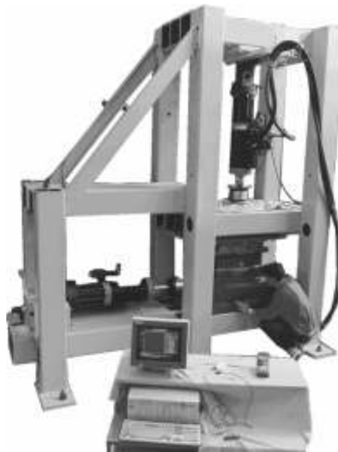
Figure 5.2: Set up of large shear box
