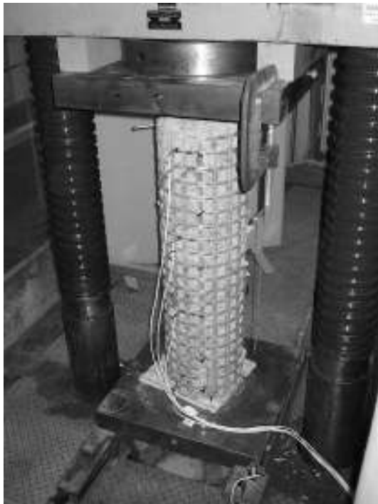
Figure 5.9: Compressive column test in Amsler apparatus
