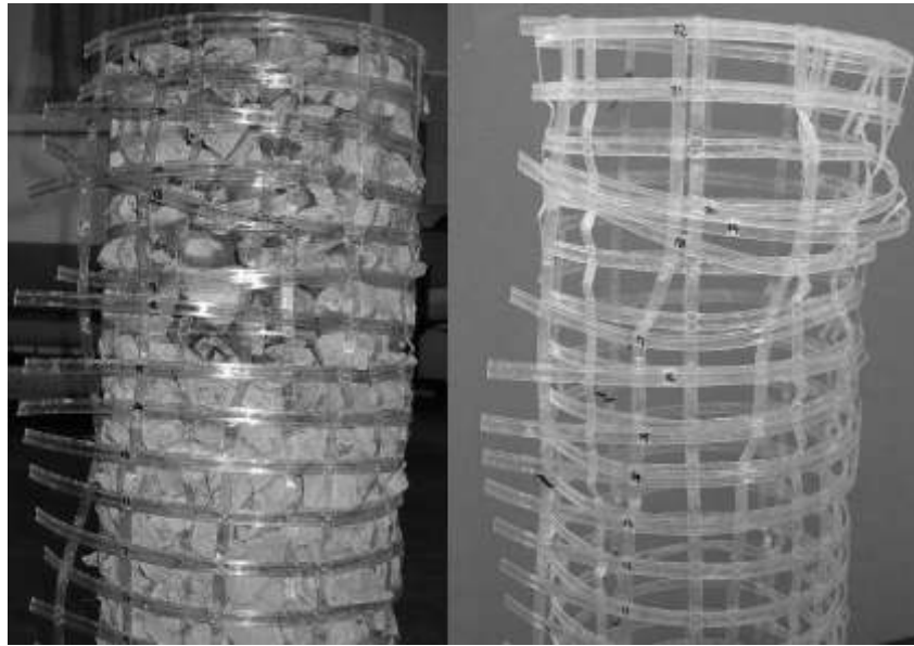
Figure 5.13: Failure mode 1 (test No. 6)
