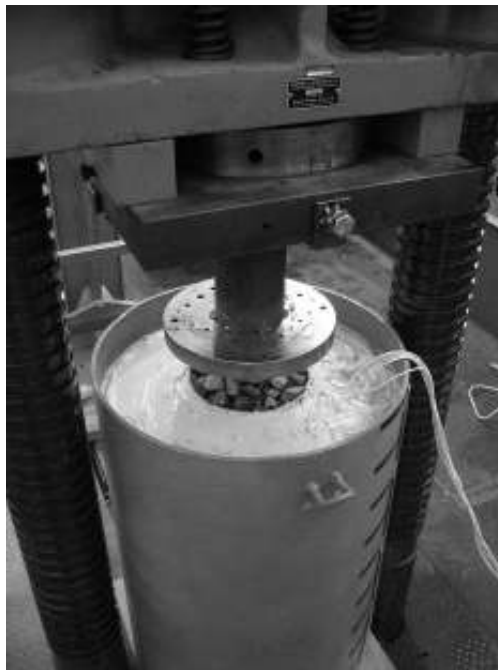
Figure 5.11: Encased column prepared for tank testing
