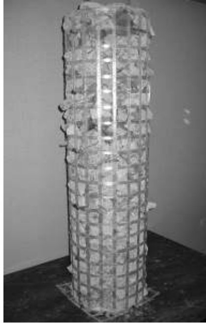
Figure 5.7: Compacted column prepared for test No.2, comprising 20/50 mm rubble
