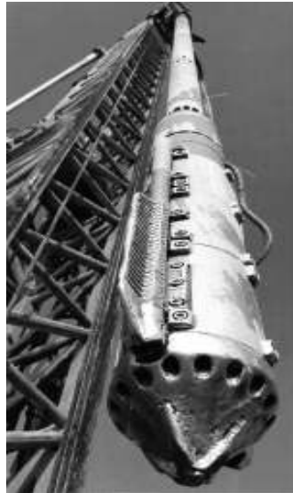
Figure 2.1: Typical vibroflot (source: Keller Grundbau GmbH)
