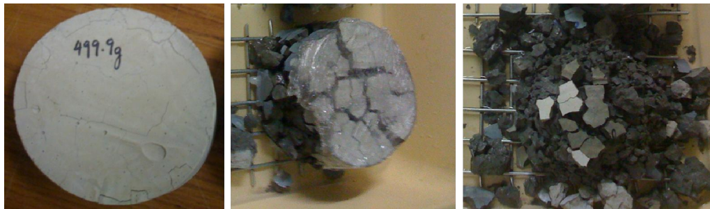
Fig. 4 OPC paste 800°C. Left, after 800°C heat treatment. Middle, immediately after water immersion. Right, few minutes after water immersion.
