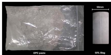
Fig. 4 OPC and 50% Slag specimens 1 year after 800°C heat treatment
