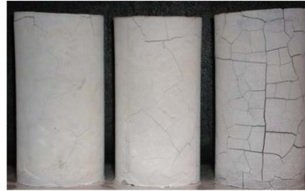
Fig. 1 Three OPC paste specimens (50 mm × 100 mm) immediately after 800°C heat treatment
