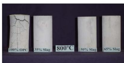
Fig. 3 Different pastes after 800°C, first day out of the furnace
