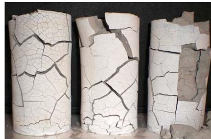
Fig. 2 Three OPC paste specimens (50 mm × 100 mm) 2 days after 800°C heat treatment
