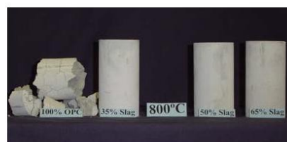
Fig. 4 Different pastes after 800°C, second day out of the furnace
