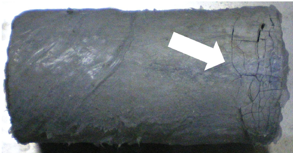
Fig. 4 Enlargement of OPC paste coated with silicone 1 week after exposure to air moisture
