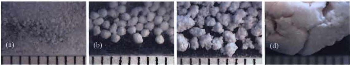
Figure 5-5 Microscopy images of (a) wetted particles and initial nuclei (b) spherical granules (c) overwetted granules and (d) cake.
