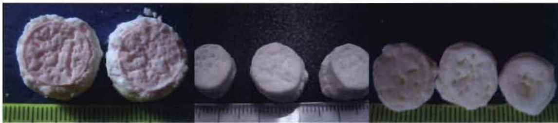
Figure 3-17 Foam created nuclei – (a) 4% HPMC on 200 mesh lactose. (b) 6% HPMC on 200 mesh lactose. (c) 3% HPC on 100 mesh lactose. Scale is in millimetres.
