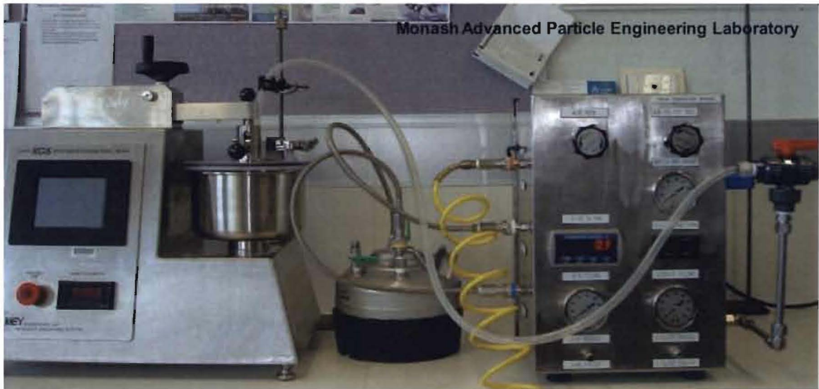
Figure 5-1 Foam granulation experimental setup – (left) high shear mixer-granulator, (middle) liquid binder storage pot and (right) foam generator.
