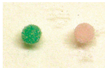
Fig. 3 A liquid marble of \text{CoCl}_2 shelled with Teflon powder changed colour after being exposed to the vapour of water-based flexographic ink (left). A fresh \text{CoCl}_2 liquid marble (right) was placed in the same Petri dish for comparison.
