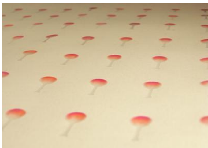
Fig. 4. Microfluidic sensor patterns are printed on an A4 sized Whatman #4 filter paper. A colorless indicator for detection of \text{NO}_2^- was also printed into the circular detection zone. Five microlitres of 5 mM \text{NO}_2^- sample solution was introduced into the channel. As the sample solution reached the detection zones of the sensors, reproducible color changes were seen.
