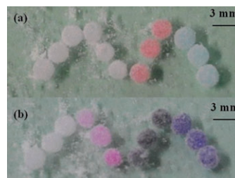
Fig. 1 (a) Four groups of liquid marbles containing water, phenolphthalein, \text{CoCl}_2 , and \text{CuCl}_2 solutions, respectively, were placed from left to right in an "M" pattern. (b) The colour changes of the indicators in these liquid marbles after exposure to ammonia gas.
