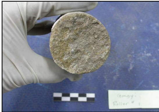
a) Cross-section of grinding mobang showing coarse-grained sandstone material (TSG R1)
