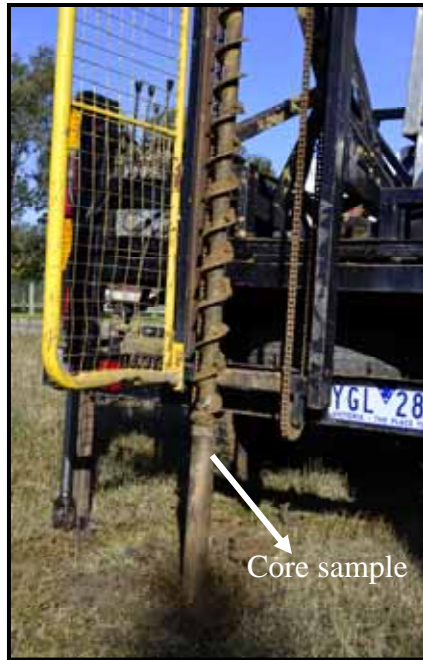
Plate 7.2. A drill-rig attached at the back of a vehicle was used to acquire 0.3 m long core sample between the depths of 1.2 – 1.5 m to provide ground truthing of geophysical data from SITE 1. Note, it is estimated that the present depth of pipeline crown is between 1-2 m.
